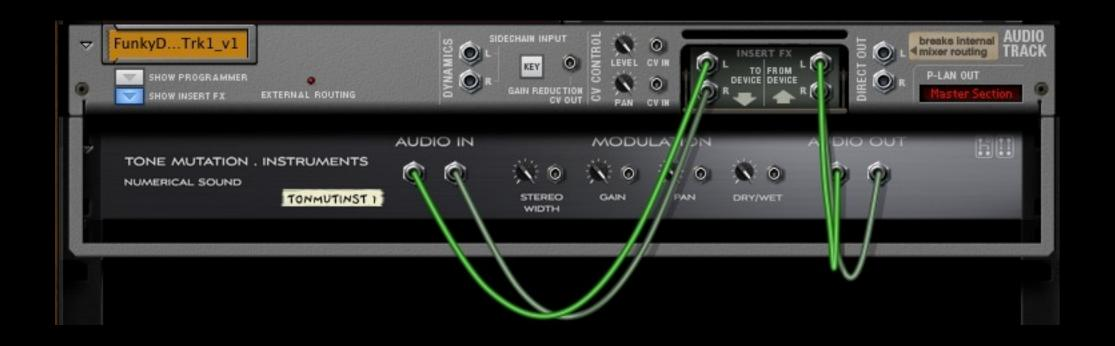
4) Program Button I (in Combinator) to act as an off/on switch for activating the TMI modules.
