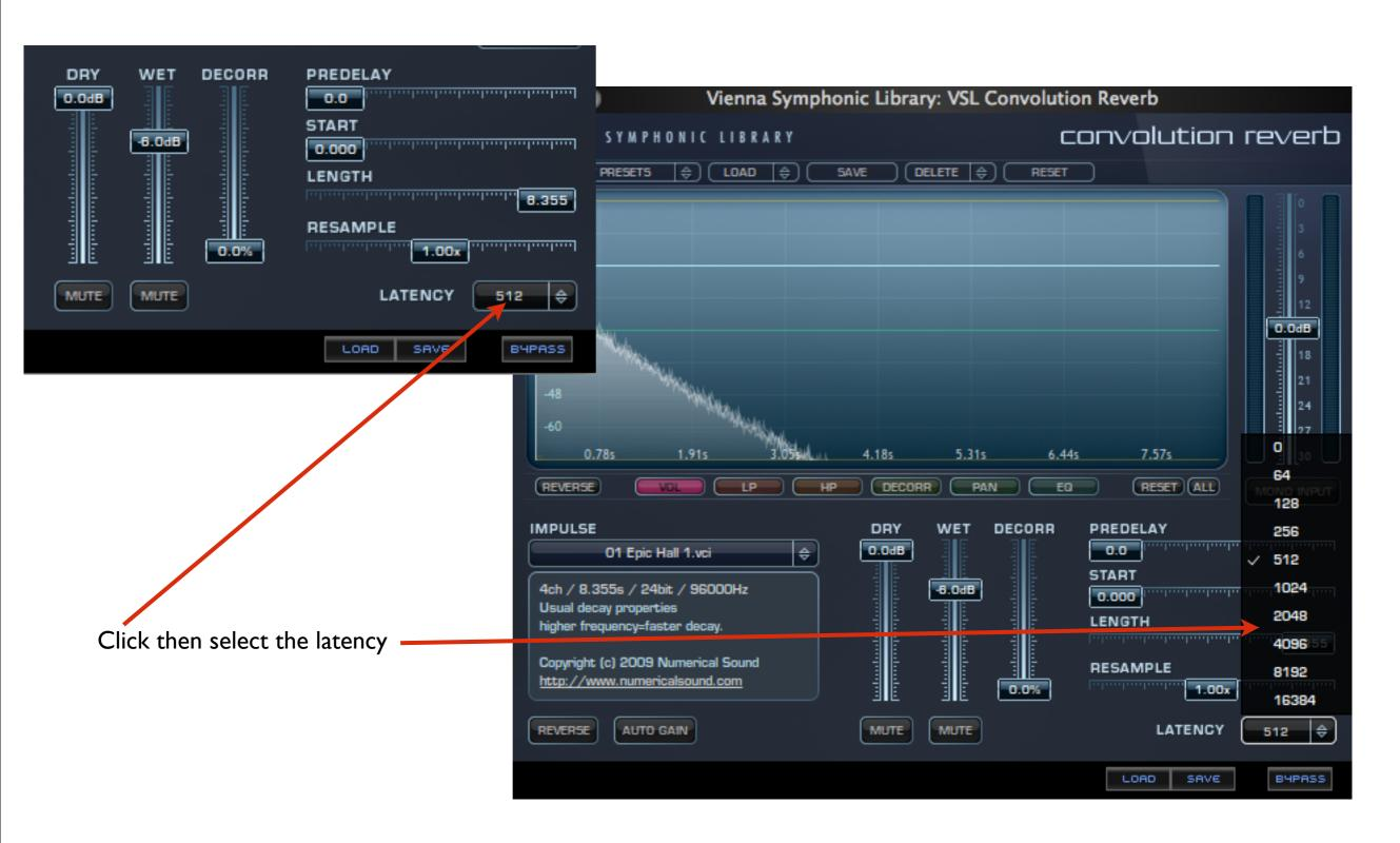
To minimize the CPU usage of the convolution plugin select a low latency value like 256-512 when adding tracks to a sequence. When you are finished editing a track you can switch to latency of 16384. This will significantly reduct the CPU usage of each VSL Convolution Plugin. For example the difference in CPU usage on a MacBook Pro from 128 samples to 16384 is 5.5X less!
